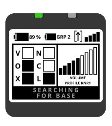
Π 89 % Battery autonomy Π **Base battery autonomy GRP 2** Sub-group selected State of isolation **Radio signal quality** Ν VOX and NOISE REDUCTION level с Volume level VOLUME Selected headset profile PROFILE RNR1 Mobile status CONNECTED TO BASE
