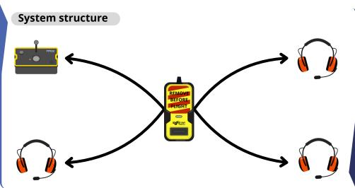
A mobile base can connect up to 4 wireless headsets, beltpacks or desktop with the pilot of the aircraft.
