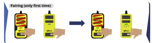
Wait 10s after power on the devices to ensure units are not already paired (devices are already connected if LEDs flash on both unit)
