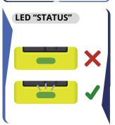
Static: no communication Flashing: communication is established
