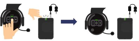
Wait 10s after power on the devices to ensure units are not already paired (devices are already connected if LEDs do not flash on both unit)
