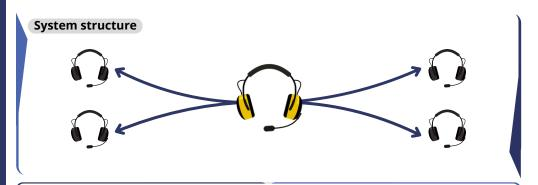
A headset to headset configuration allows up to 4 wireless units to be connected to a master headset.
