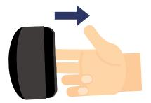
Remove the ear pads by pulling it straight out.
