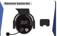
Replace batteries by opening the black hood with your thumb. Remove batteries by pulling the tape.
